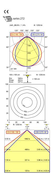
Light source LED Work equipment Without Connected load 230 V; AC; 50 Hz; 60 Hz **Power consumption** ca. 16 W Luminous flux approx. 1.250 lm **Luminous efficiency** approx. 78 lm/W Light type/-color Cold white Colour temperatur approx. 5.000 K CRI ≥ 80 Color rendering index **Light distribution** Direct **Direct ratio** approx. 99 % 100° Beam angle **Chromaticity tolerance LED** < 4 SDCM
