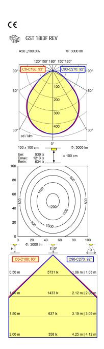
Light source LED Work equipment Power supply unit 220 - 240 V; AC; 50 Hz; 60 Hz **Connected load Power consumption** ca. 35 W approx. 3.000 lm Luminous flux Light type/-color Cold white Colour temperatur approx. 5.000 K Color rendering index CRI ≥ 80 Direct
