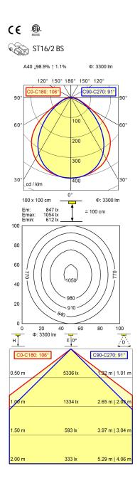
Light source LED Work equipment Without 22 - 26 V; DC **Connected load Power consumption** ca. 44 W Luminous flux approx. 3.300 lm **Luminous efficiency** approx. 75 lm/W Light type/-color Cold white approx. 5.000 K Colour temperatur CRI ≥ 80 Color rendering index **Light distribution** Direct **Direct ratio** approx. 99 % 100° Beam angle
