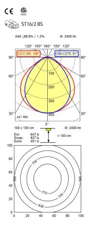
Light source LED Work equipment Without 22 - 26 V; DC **Connected load Power consumption** ca. 31,5 W Luminous flux approx. 2.400 lm **Luminous efficiency** approx. 75 lm/W Light type/-color Cold white Colour temperatur approx. 5.000 K CRI ≥ 80 Color rendering index **Light distribution** Direct **Direct ratio** approx. 99 % 100° Beam angle **Chromaticity tolerance LED** < 4 SDCM Glare control Diffuser foil Luminance (L65)  $\leq 14.000 \text{ cd/m}^2$
