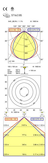
Light source LED Work equipment Without 22 - 26 V; DC Connected load **Power consumption** ca. 25 W Luminous flux approx. 1.900 lm **Luminous efficiency** approx. 76 lm/W Light type/-color Cold white approx. 5.000 K Colour temperatur CRI ≥ 80 Color rendering index **Light distribution** Direct **Direct ratio** approx. 99 % 100° Beam angle **Chromaticity tolerance LED** < 4 SDCM Luminance (L65)  $\leq 13.000 \text{ cd/m}^2$ System of protection IP 67
