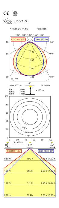
Light source LED Work equipment Without **Connected load** 22 - 26 V; DC **Power consumption** ca. 12,5 W Luminous flux approx. 950 lm **Luminous efficiency** approx. 73 lm/W Light type/-color Cold white Colour temperatur approx. 5.000 K CRI ≥ 80 Color rendering index Light distribution Direct **Direct ratio** approx. 99 % 100° Beam angle **Chromaticity tolerance LED** < 4 SDCM Glare control Diffuser foil Luminance (L65)  $< 12.000 \text{ cd/m}^2$ Unified glare rating (4H 8H) ≤ 25
