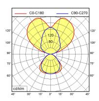
Work equipment Electronic ballast Connected load 220 - 240 V; 50 Hz; 60 Hz **Power consumption** ca. 49 W Standby ca. 0,3 W Power factor env. 0,950 Luminous flux approx. 7.000 lm Luminous efficiency approx. 142 lm/W Light type/-color Cold white approx. 4.000 K Colour temperatur Color rendering index CRI ≥ 80 **Light distribution** Direct/indirect **Direct ratio** approx. 34 %
