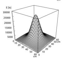
Light sourceLEDWork equipmentWithoutConnected load22 - 26 V; DCPower consumptionca. 5 WLuminous fluxapprox. 490 lmLight type/-colorCold whiteColour temperaturapprox. 5.000 K
