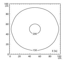
Light source LED Work equipment Without 16 - 32 V; DC **Connected load Power consumption** ca. 8,5 W approx. 940 lm Luminous flux Light type/-color Daylight Colour temperatur approx. 5.400 K Color rendering index CRI ≥ 80 **Light distribution** Direct **Direct ratio** approx. 83 % Beam angle >120° **Chromaticity tolerance LED** < 5 SDCM Glare control Without Luminance (L65)  $\leq 4.000 \text{ cd/m}^2$ Unified glare rating (4H 8H) ≤ 22
