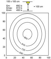
Light sourceLEDWork equipmentWithoutConnected load22 - 26 V; DCPower consumptionca. 32 WLuminous fluxapprox. 2.280 lmLuminous efficiencyapprox. 71 lm/W
