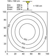
Light sourceLEDWork equipmentWithoutConnected load22 - 26 V; DCPower consumptionca. 16 WLuminous fluxapprox. 1.140 lm
