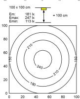
Light sourceLEDWork equipmentWithoutConnected load22 - 26 V; DCPower consumptionca. 8 WLuminous fluxapprox. 570 lmLuminous efficiencyapprox. 71 lm/W
