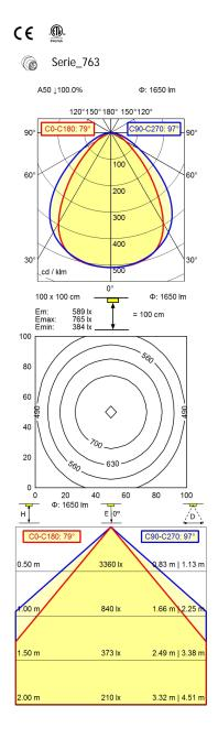
LED light source work equipment without connected load 18 - 30 V; direct current (DC) power consumption ca. 18 W luminous flux approx. 1.650 lm luminous efficiency approx. 91 lm/W light type/-color cold white colour temperatur approx. 5.000 K color rendering index CRI ≥ 80 light distribution direct; symmetric
