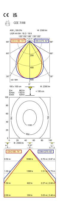
Light source LED Work equipment Electronic ballast **Connected load** 220 - 240 V; AC; 50 Hz; 60 Hz **Power consumption** ca. 26 W Luminous flux approx. 2.300 lm Luminous efficiency approx. 88 lm/W Light type/-color Daylight Colour temperatur approx. 6.500 K Color rendering index  $CRI \ge 90; R9 \ge 50$ **Light distribution** Direct; Symmetric **Direct ratio** approx. 100 % Beam angle 75%
