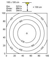
Light sourceLEDWork equipmentWithoutConnected load22 - 26 V; DCPower consumptionca. 25 WLuminous fluxapprox. 1.880 lmLuminous efficiencyapprox. 75 lm/W
