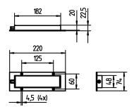
Light source LED Work equipment Without 20 - 28 V; DC **Connected load Power consumption** ca. 6 W approx. 400 lm Luminous flux Light type/-color Cold white Colour temperatur approx. 5.000 K Color rendering index CRI ≥ 80 Light distribution Direct; Symmetric Glare control Without
