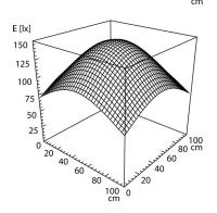
Light source LED Work equipment Without 20 - 28 V; DC **Connected load Power consumption** ca. 6 W approx. 400 lm Luminous flux Light type/-color Cold white Colour temperatur approx. 5.000 K Color rendering index CRI ≥ 80
