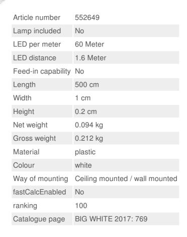
Flexible, 24V DC LED RGB strip whose rear side is fitted with adhesive tape for simple installation. The electrical connection of the strips, which come in several lengths, is done to a compatible 24V DC voltage power supply. Feed-in cables, direct connectors, flexible and corner connectors are available as further accessories. In addition, the strip comes in various lengths. A separate controller is needed to control the RGB effects.
