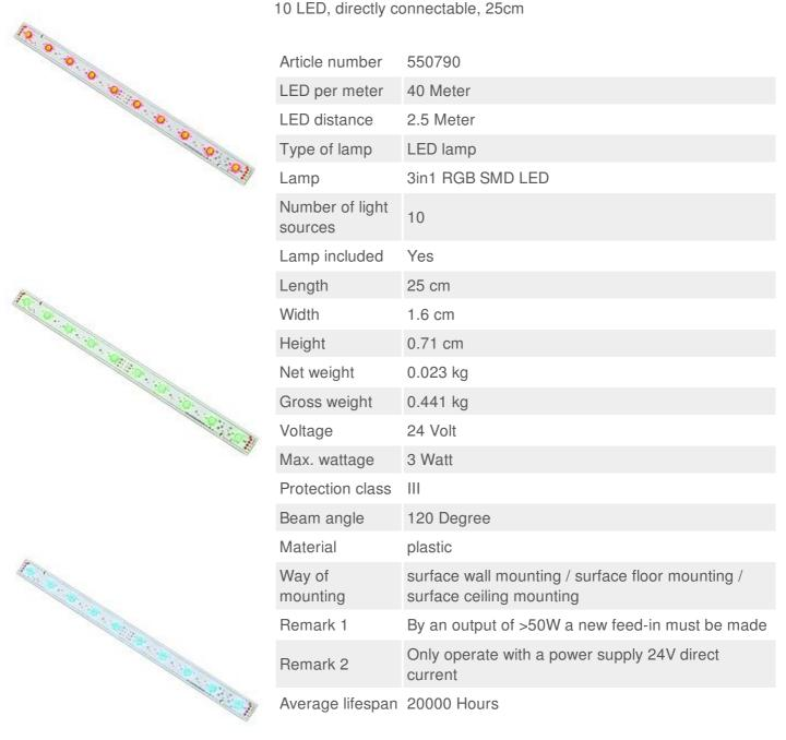
A rigid 24V DC LED RGB strip to be connected to a RGB controller. With the incorporated 3in1 RGB LED, the colours are mixed directly at the diode. The requested colour is shown immediately. On accessory we offer connection leads, flex-connectors, mounting tracks and clips.
