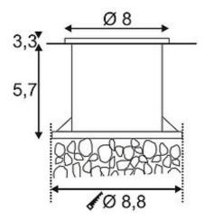
The low-voltage recessed ground luminaire with round stainless steel bezel and frosted glass cover is equipped with several LED. The fitting is available in different colour versions and rated IP67 making it suitable for outdoor use. A suitable toroidal transformer providing 12V alternating current is required for operation. A suitable installation for simplified mounting is included. This luminaire contains built-in LED lamps. EEK: A - A++. The lamps cannot be changed in the luminaire.
