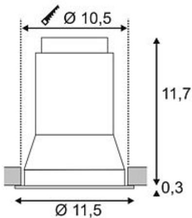
The DIVIS GU6.5 downlight in round shape with glass cover is equipped with a GU6.5 lampholder for metal halide lamps of the same type. Suitable reflectors with different beam angles are available as optional accessory. Available in the colours white and silvergrey, with higher or lower reflector position, a suitable and lamp related ballast is required for operation of DIVIS GU6.5. This luminaire is compatible with bulbs of the energy classes: A - A+
