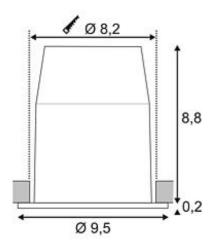
The rigid LED spotlight HORN LED is made from aluminium and is the LED lighting solution for applications where flooding illumination and low installation depths are required. The 3W Power LED in warmwhite light colour provides the necessary illumination intensity. Available in two different colour versions, a suitable constant current driver providing 700mA is required for operation. This luminaire contains built-in LED lamps. EEK: A - A++. The lamps cannot be changed in the luminaire.
