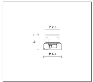
3 MODULES LED RGB 24V PWM Rated luminaire luminous flux: 53lm
