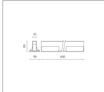
MODULES LED 3000K 24V 360lm CRI 80 Rated luminaire luminous flux: 165lm
