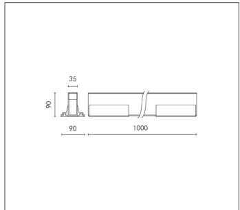
MODULES LED 3000K 24V 740lm CRI 80 Rated luminaire luminous flux: 330lm
