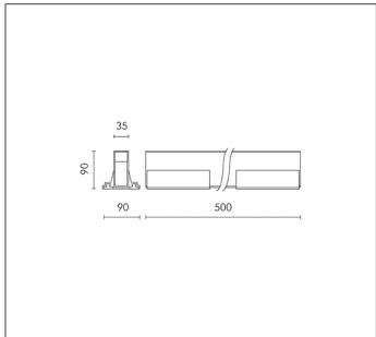
MODULES LED 4000K 24V 389lm CRI 80 Rated luminaire luminous flux: 109lm
