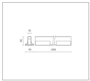
MODULES LED 4000K 24V 799lm CRI 80 Rated luminaire luminous flux: 218lm
