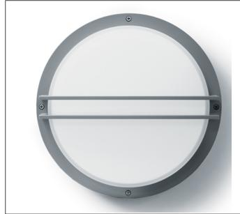
MODULES LED 4000K 230V 2106lm CRI 90 MacAdam step 3 Rated luminaire luminous flux: 1063lm Rated input power: 22W Luminaire efficacy: 48lm/W Electronic ballast 230V 0/50/60Hz
