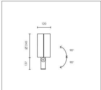
HIT-TC CRI 70W CLEAR G8,5 6600lm Rated luminaire luminous flux: 3432lm
