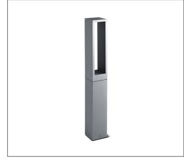
MODULES LED 4000K 230V 1048lm CRI 90 MacAdam step 3 Rated luminaire luminous flux: 421lm Rated input power: 13W Luminaire efficacy: 32lm/W Electronic ballast 220÷240V 0/50/60Hz
