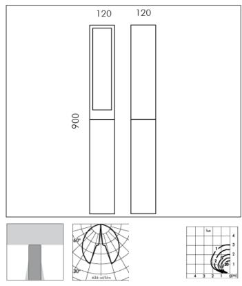
\* Photometric measured using WHITE LED 3000K
