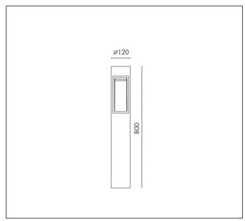
HIT-TC CE 20W PGJ5 1700lm Rated luminaire luminous flux: 221lm
