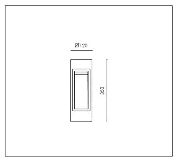
4 MODULES LED 6000K 230V CRI 75 Rated luminaire luminous flux: 141lm
