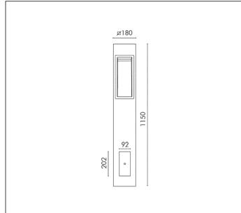
HIT-TC CE 35W G8,5 3300lm Rated luminaire luminous flux: 594lm
