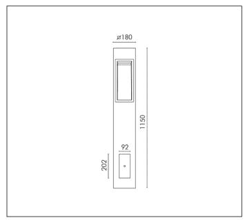
10 MODULES LED 6000K 230V CRI 75 Rated luminaire luminous flux: 534lm
