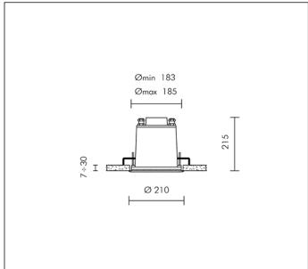
TC-TEL 18W Gx24q-2 1200lm Rated luminaire luminous flux: 348lm
