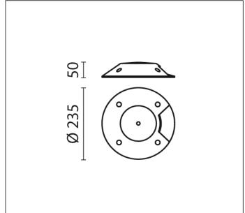
MODULES LED 3000K 230V CRI 80 Rated luminaire luminous flux: 65lm Rated input power: 3.6W
