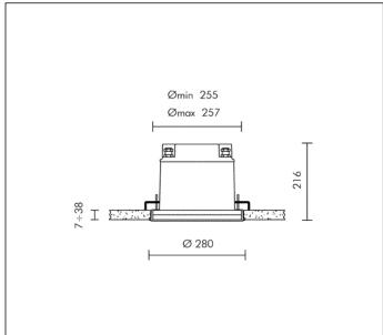
HIT-CRI 70W CLEAR G12 6600lm Rated luminaire luminous flux: 3533lm
