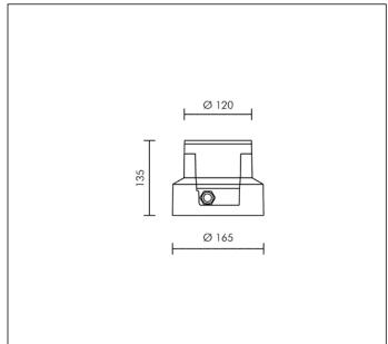
3 MODULES LED RGB 24V PWM Rated luminaire luminous flux: 5lm
