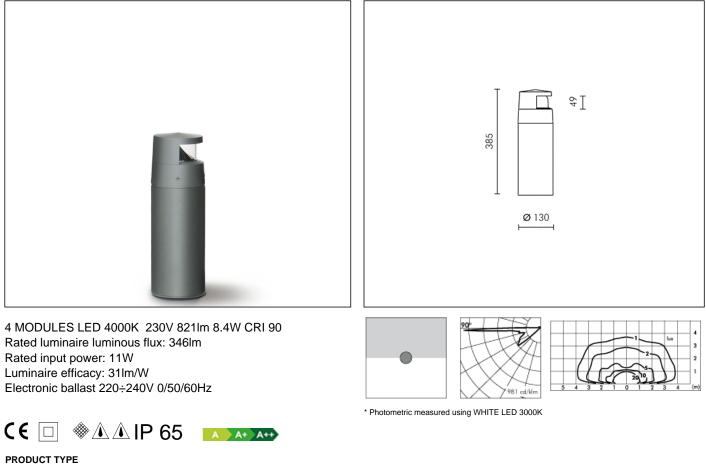
Bollard fitting. IP rating IP 65 MATERIAL CHARACTERISTICS
