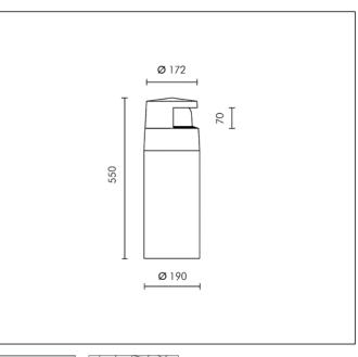
1 MODULES LED COB 4000K 1792lm CRI 90 Rated luminaire luminous flux: 658lm Rated input power: 18W Luminaire efficacy: 37lm/W Electronic ballast 220÷240V 50/60Hz
