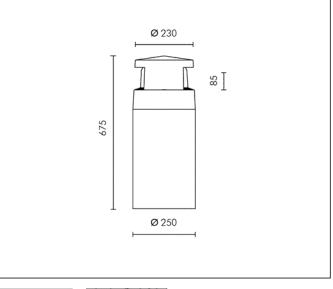
1 MODULES LED COB 4000K 3801Im CRI 90 Rated luminaire luminous flux: 955Im Rated input power: 38W Luminaire efficacy: 25Im/W Electronic ballast 220÷240V 0/50/60Hz
