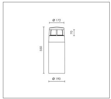
HIT-TC CRI 20W G8,5 1700lm Rated luminaire luminous flux: 510lm
