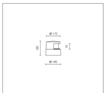
HIT-TC CRI 20W G8,5 1700lm Rated luminaire luminous flux: 272lm
