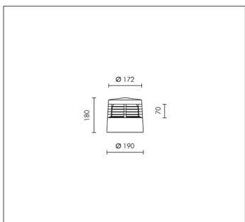
TC-TEL 18W Gx24q-2 1200lm Rated luminaire luminous flux: 180lm
