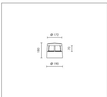
TC-TEL 18W Gx24q-2 1200lm Rated luminaire luminous flux: 360lm
