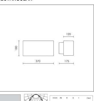
MODULES LED 4000K 2009Im CRI 90 Rated luminaire luminous flux: 1254Im Rated input power: 26W Luminaire efficacy: 48Im/W Electronic ballast 220÷240V 0/50/60Hz
