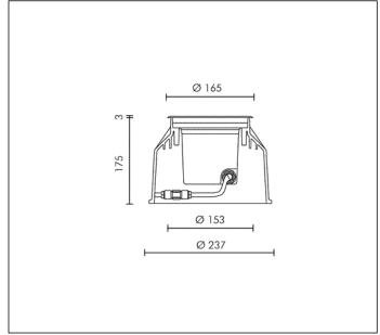
MODULES LED RGB 24V PWM 390lm Rated luminaire luminous flux: 19lm
