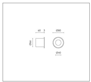
MODULES LED 6000K 230V CRI 75 Rated luminaire luminous flux: 40lm Rated input power: 1W Luminaire efficacy: 40lm/W
