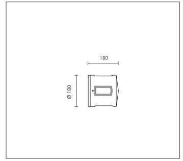
HIT-TC CRI 35W G8,5 3300lm Rated luminaire luminous flux: 429lm
