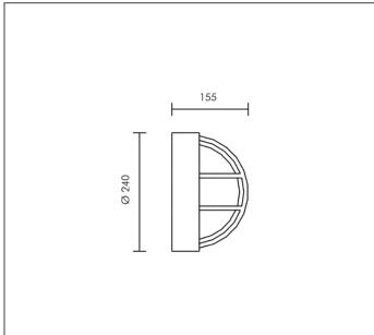
TC-DEL 18W G24q-2 1200lm Rated luminaire luminous flux: 588lm
